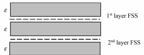
(b) Double layer FSS with dielectric support
